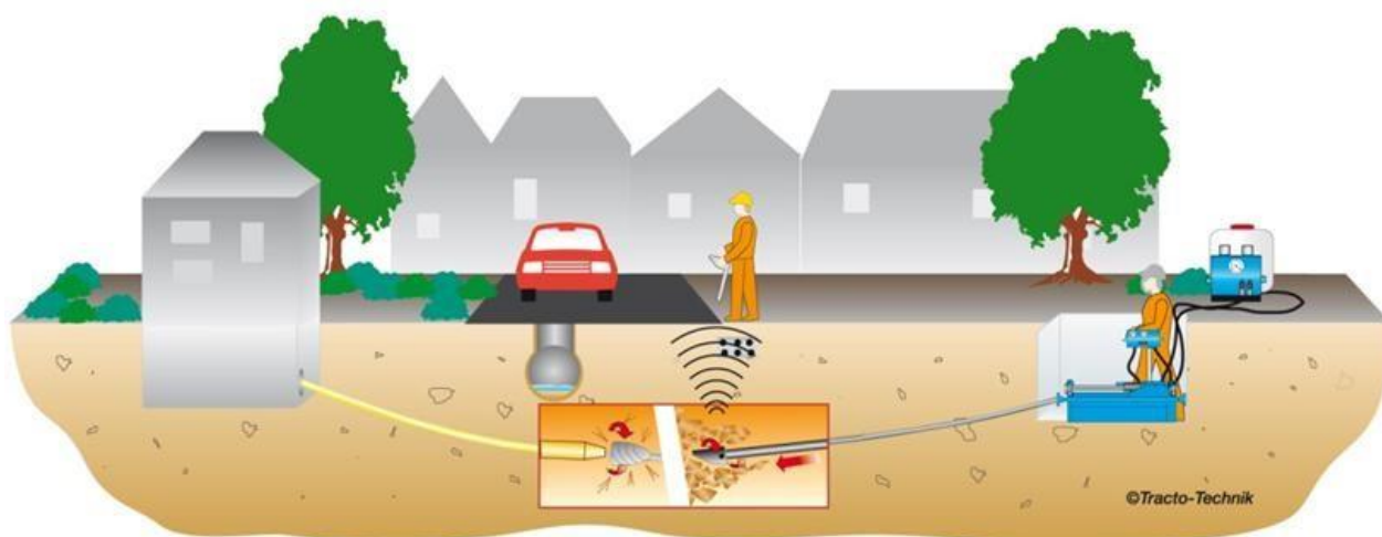
Figur 1. Illustration af styret underboring
